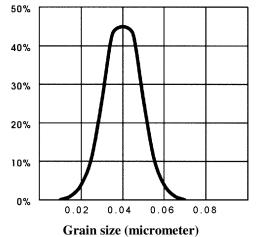
Figure 3: Grain Size distribution curve for VRP-M.
