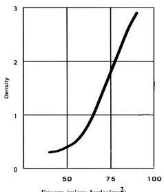
**Energy (micro Joules/cm<sup>2</sup>)** Figure 2: Characteristic curve for VRP-M
