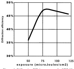
Figure 4: Diffraction Efficiency curves for VRP-M
